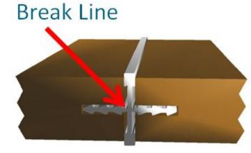
MCLIN-Cap MCLIN-Corner MCLIN-Join The Cap and the Join have break lines at the base of the fir tree. This enables sections of the fir tree to be cut then by bending back and forth, broken off.
