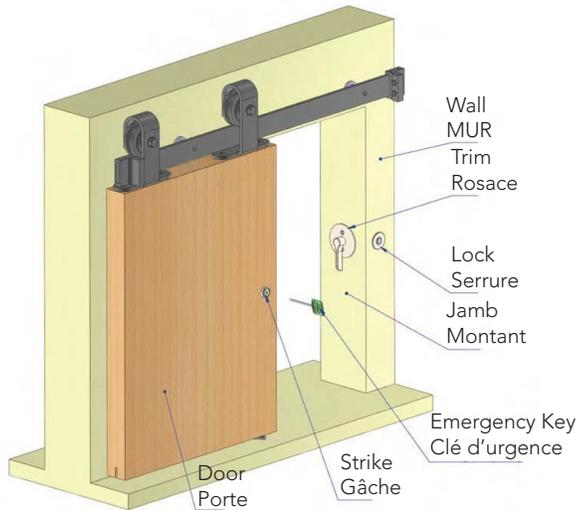
Installation based on barn door application where doors are hung on the OUTSIDE of the room.
