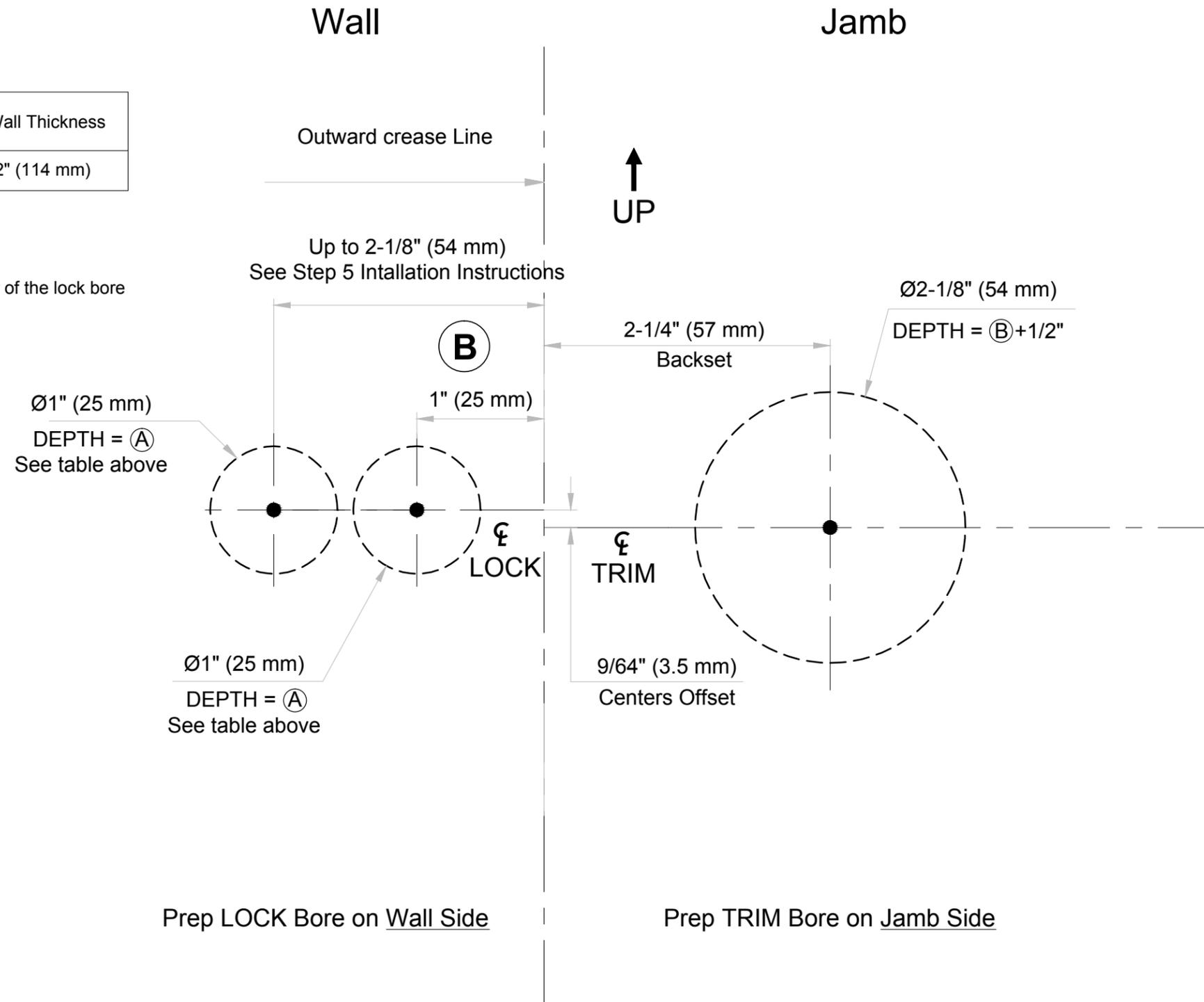
Template Dimensions do NOT provide allowances for gaps between wall studs and drywall.
