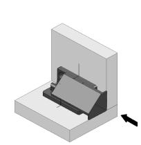
Key being installed in other end of the assembled Hooks.
