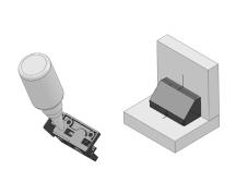
An alternative to marking screw locations is to apply glue to the mounting faces of the Hooks to aid placement. Line up notches in the Hooks with the marked lines then press and hold the assembled 90D in place. Allow time for glue to dry.
