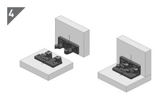
After all screws are in place, bring the two substrates together. The two sets of Hooks will self-align as shown.
