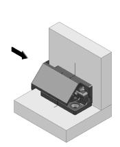
Install the Key remembering it only needs to travel 1 pitch for full engagement. Use the padlock symbol as a guide. The Key is also bidirectional and can be installed either end, see step 5b.
