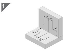
Mark center line on both substrates. Mark mounting screw center points by measuring or place product in position and mark.
