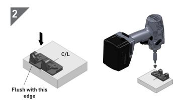
Orientate and fasten each Hook with 2 x 8G screws. Ensure sufficient screw embedment in substrate. Align center line on hook to center line on substrate. Keep Hook flush with edge indicated.
