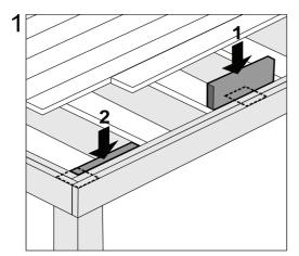
1. Add additional blocking as needed to accept all four screws and center lag screw.
