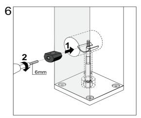
**6.** Finally install the gear housing onto the screw shaft, tighten using a 6mm hex bit (provided) in a power or hand tool. Finish off with a wood plug (not included) as needed or slide post cover over wood post at this point.
