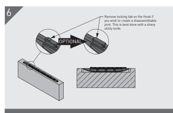
After glue is applied, insert Hook into slot until flush with substrate. Allow to dry as per glue manufactures instructions.
