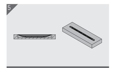
After glue is applied, insert Key into slot until flush with substrate. Allow to dry as per glue manufactures instructions.
