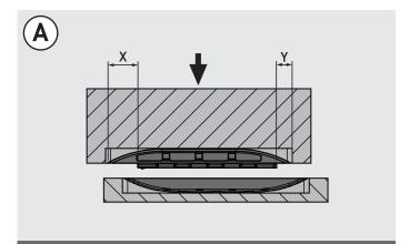
Note the offset of the lugs on the Hook body, length X is larger than Y. Insert the Hook into the Key with the longer X end towards the face to be pushed during assembly.
