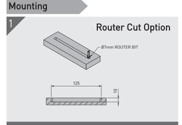
Use a Ø7mm router bit to cut a slot in both substrates where the Hook and Key of the Mini 120 is to be mounted. Depth needs to be 10mm for each.
