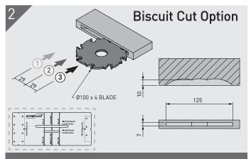
Set the depth stop to #20 and guide height for substrate thickness. Plunge in 3 locations then repeat using the **Mark-Out Template**, packing the guide 3mm to achieve a 7mm cut.
