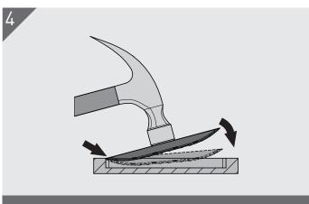
To aid in the installation of the Key and Hook, start by inserting one end in the slot when use a hammer or mallet to tap the component into place.
