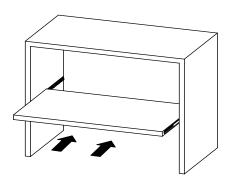
Insert shelf and push in until locked in position and flush with front edge.
