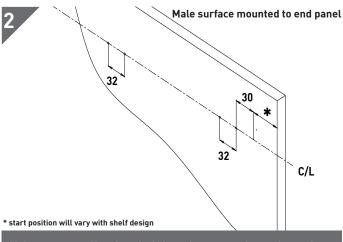
Using a center line for shelf location, on end panel, mark the starting position (\*). Next mark 30mm to the first set of holes as shown above. The position of the second set of holes will be dermind by the depth of the shelf.
