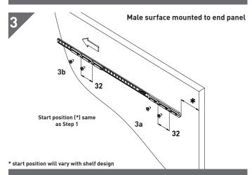
3a. First fix the male strap in place with screws, using the marked center line.
