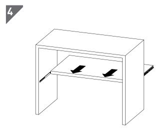
Insert shelf from back and push forward until locked in position and flush with front edge of frame.
