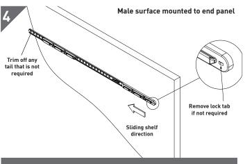
Remove locking tab if not required and trim off the excess strap that protrudes past the end of the panel.
