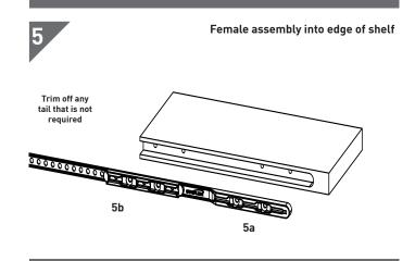
5a. Screw the female strap in place in the routed edge of the shelf. (Pilot holes are recommended for all screws).
