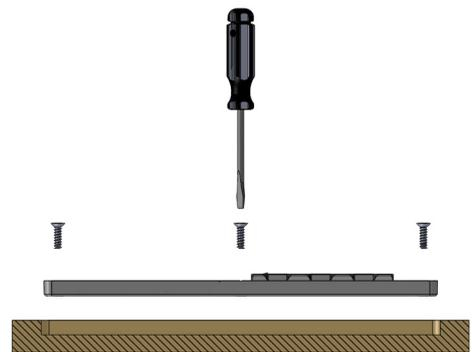
Place the 1st Megalox into slot ensure flush with substrate. Pilot drill screw position, use x 3 8G countersunk screws, Euro screws or simply glue into position using Liquidlox.
