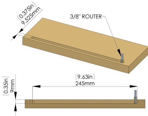
Use a 9.525mm (3/8") router bit to cut a slot in both substrates to correct length. Depth needs to be 9mm.
