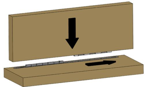
Complete the installation by sliding fully to lock up position. Remember to remove locking tab if applicable.
