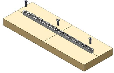
Place Megalox onto surface in position and pilot drill screw position use 3x 8G countersunk screws or Euro screws.
