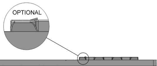
Megalox is either permanent or reusable, simply remove locking tab using blade or sander to disassemble.
