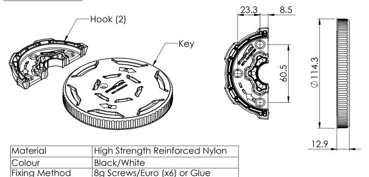
\*Ensure sufficient screw embedment in substrate
