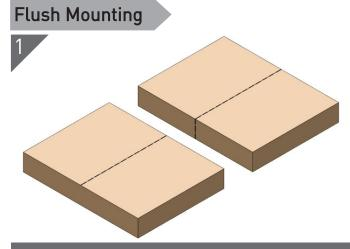
Position 2 surfaces tight together into position, mark out a centreline on both surfaces.
