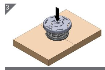
Locking tabs can remain in place, this is the final locking positions.
