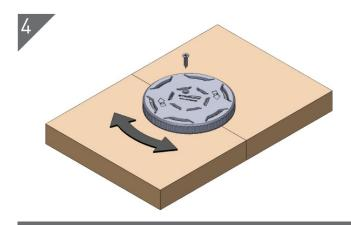
Join 2 surfaces together then place key over the top, push down and turn until locked.
