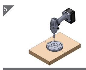
For permanent lockup use a screw position in key ensuring enough embedment into substrate.
