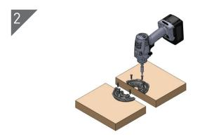
Position 1st half of 180D flush with edge of substrate (note position lug will be slightly proud) ensure main face is flush across the full edge using centreline position and screw into position.
