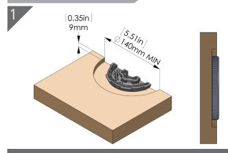
Router position at centrelines into 2 surfaces at current depth 9mm, either circular or square cut ensure sufficient clearance for key to lock down and turn.
