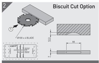
Set the depth stop to #20 and guide height for substrate thickness. Plunge in once then repeat using the **Mark-Out Template**, packing the guide 3mm to achieve a 7mm cut.
