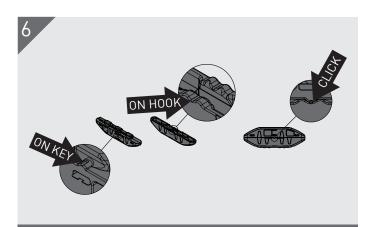
The Mini 60 features locating tabs which click into place when fully assembled. Please note this feature is not a lock, making the joint fully reversible.
