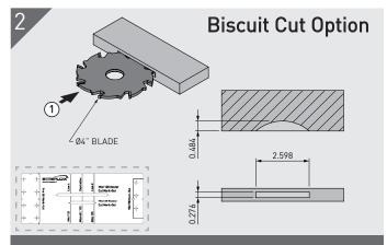
Set the depth stop to #20 and guide height for substrate thickness. Plunge in once then repeat using the **Mark-Out Template**, packing the guide 0.118" to achieve a 0.276" cut.
