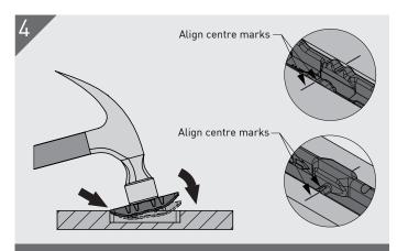
To aid in the installation of the Key and Hook, start by inserting one end in the slot when use a hammer or mallet to tap the component into place. Ensure center lines on substrate align with center marks on Hook and Key.
