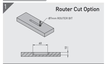
Use a Ø7mm router bit to cut a slot in both substrates where the Hook and Key of the Mini 60 is to be mounted. Depth needs to be 10mm for each.
