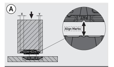
Note the offset of the lugs on the Key body, length X is larger than Y. Insert the Hook into the Key with the longer X end towards the face to be pushed during assembly.
