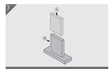
Assembly components remembering the Key only needs to travel 1 pitch for full engagement. This is detailed in steps A and B.
