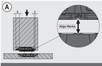
Note the offset of the lugs on the Key body, length X is larger than Y. Insert the Hook into the Key with the longer X end towards the face to be pushed during assembly.
