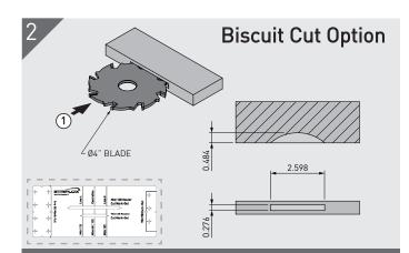
Set the depth stop to #20 and guide height for substrate thickness. Plunge in once then repeat using the **Mark-Out Template**, packing the guide 0.118" to achieve a 0.276" cut.
