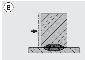
To complete the assembly push the end of the substrate (with X offset) until the Mini 60 is fully engaged.
