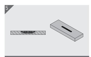
After glue is applied, insert Key and Hook into slot until flush with substrate. Allow to dry as per glue manufactures instructions.
