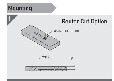
Use a Ø9/32" router bit to cut a slot in both substrates where the Hook and Key of the Mini 60 is to be mounted. Depth needs to be 0.394" for each.
