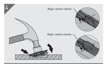
To aid in the installation of the Key and Hook, start by inserting one end in the slot when use a hammer or mallet to tap the component into place. Ensure center lines on substrate align with center marks on Hook and Key.
