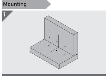
Mark center line on both substrates. The 90D 98 works on box joints (shown), t-section and mitered joints. Mark mounting screw centre points by measuring or with the aid of the **Mark-Out Template**.
