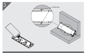
An alternative to marking screw locations is to apply glue to the mounting faces of the Hooks to aid with placement. Line up notches in the Hooks with the marked lines them press and hold the assembled 90D in place. Allow time for glue to dry.
