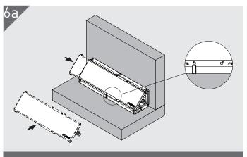
Install the Key remembering it only needs to travel 1 pitch for full engagement. Use the padlock symbol as a guide. The Key is also bidirectional and can be installed either end, see step 6b.
