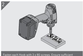
Fasten each Hook with 3 x 8G screws. Ensure sufficient screw embedment in substrate.
