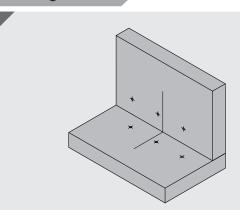
Mark center line on both substrates. The 90D 98 works on box joints (shown), t-section and mitered joints. Mark mounting screw centre points by measuring or with the aid of the **Mark-Out Template**.
