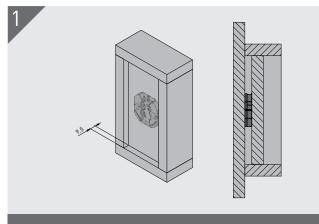
Setting back the mounting face of either the Hook (as shown) or Key by 9.5mm results in a concealed joint without the need to cut rebates.
