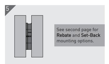
When assembled, the substrates will be separated by the thickness of the engaged Clip 50.
