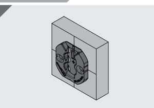
Mark center lines, vertical and horizontal, on both substrates. Flush mounting requires no additional preparation. Line the notches in each component (Hook shown here) with the center lines. **Mark-Out Template** can also be used.
