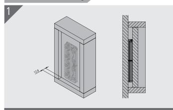
Setting back the mounting face of either the Hook (as shown) or Key by 12.8mm results in a concelled joint without the need to cut rebates.
