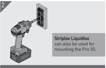
Hold the component in place and fasten to the substrate with  $8 \times 8G$  screws. Repeat for matching component. Ensure sufficient screw embedment in substrate.
