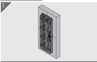
Mark center lines, vertical and horizontal, on both substrates. Flush mounting requires no additional preparation. Line the notches in each component (Hook shown here) with the center lines. Mark-Out Template can also be used.
