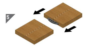
Position both surfaces together aligned and move together to form joint.(180 degree, T Joint, Box joint and Mitre joints).
