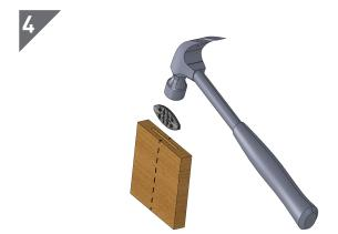
Position Biscuit at centreline and knock in with hammer. Unique grips will hold in place (no glue required). Glue may be used (CA). Glue will travel into void areas.
