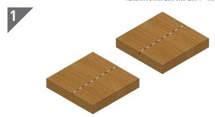
Mark out position on both surfaces to align.
