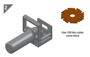
Set depth stop to #20 on Biscuit Cutter/ Plate Joiner and plunge in on centreline position or cut position with router using 4mm bit.
