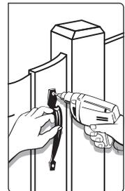
**Gate Pull Installation:** Mark screw locations. Drill pilot holes. Fasten screws.
