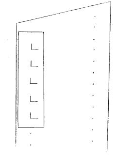
5. Rotate the rack horizontally so the rear of the rack is on the rear side of the closet. Extend the rack to the front so the rear screw slot on the slide is fully exposed. Secure the screw slot to the rear screw hole on the closet by a provided screw.
