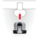
Assembling with threaded pin to achieve horizontal connection
