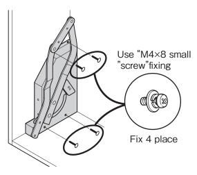
**4.** Install "Connection Bar" to both side of the structure parts.
