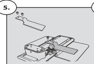
Attach the actuator handle as shown using the M5x12mm screws.
