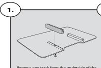
Remove one track from the underside of the work surface and set aside.
