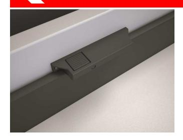
This drawer latch locks the inner top drawer when you open the door. A simple touch on the top of the latch releases the top drawer to give access to the bottom one.
