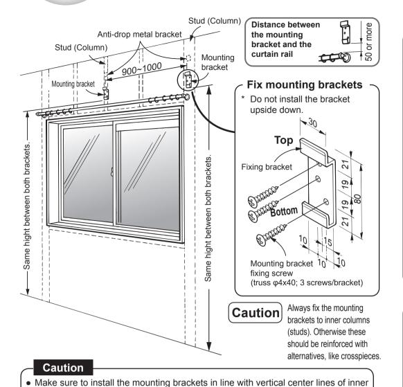
Two mounting brackets should be positioned at the same height against the floor.
