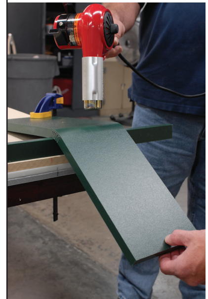
Using a heat gun to bend around a large radius takes time and should not be rushed.
