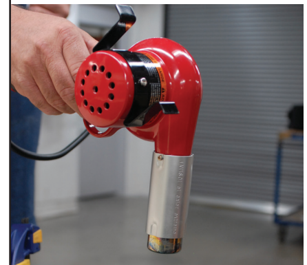
Heat guns can be used to bend King StarBoard® ST around a radius.
