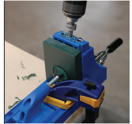
Make sure to pilot hole and counterbore or countersink all screws.
