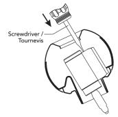
Alternatively, knock the cylinder with a screwdriver to push knob cap out as shown.
