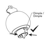
Compress the sides, force dimples open and pull knob cap.
