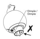
Do not compress dimple. This will cause the dimple to snap more tightly on the knob.
