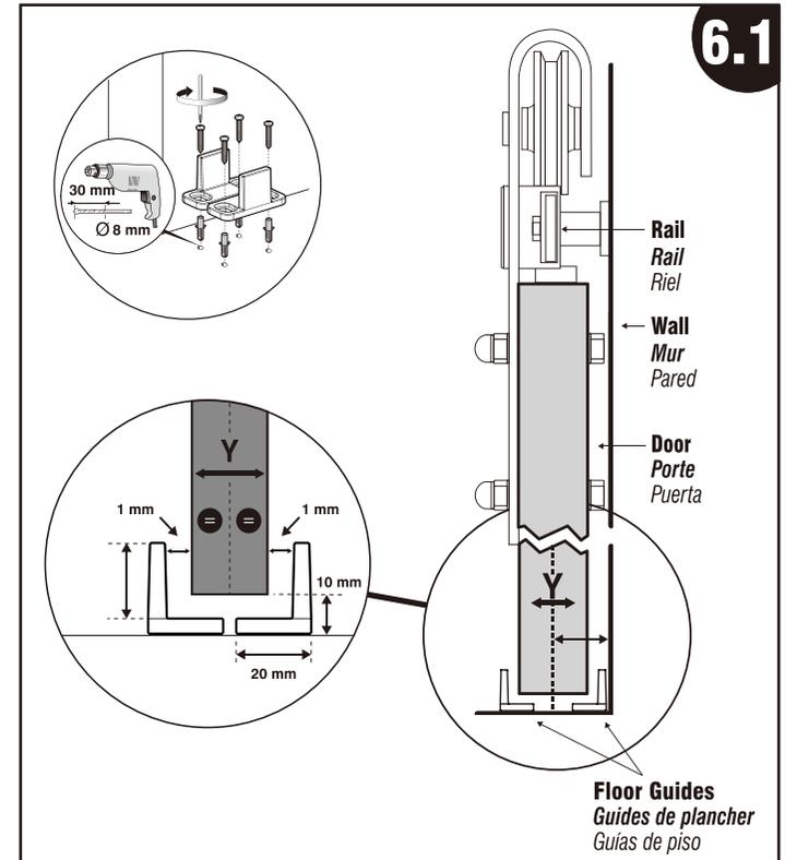
**6.1 Visible floor guides – Door without bottom groove**
