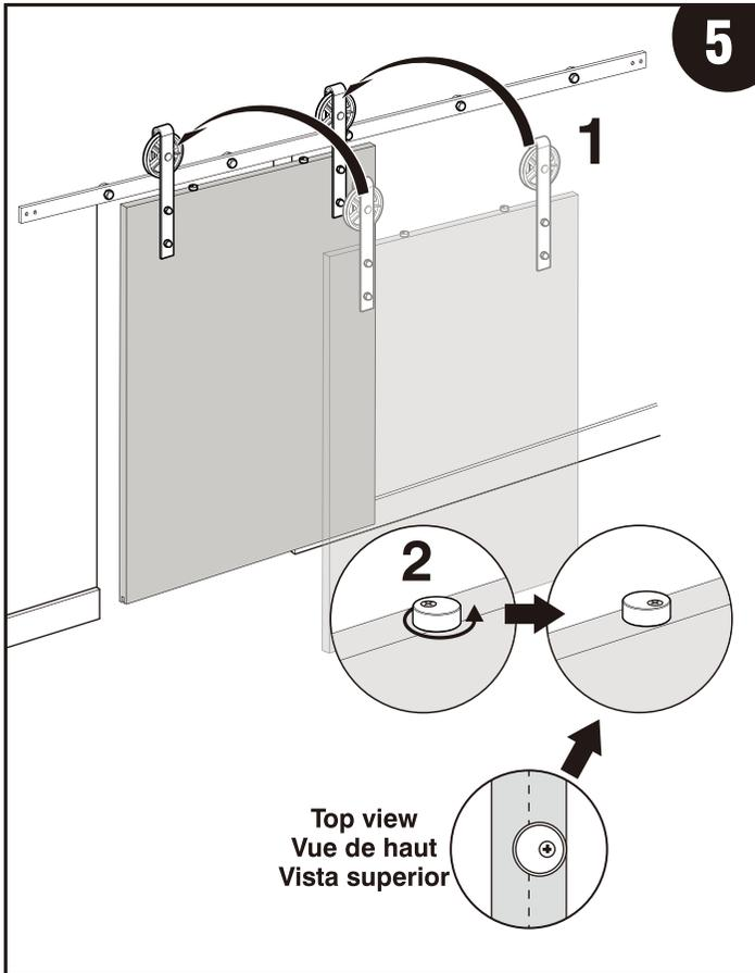
**Step 5: Install the door and adjust jump-proof devices**
