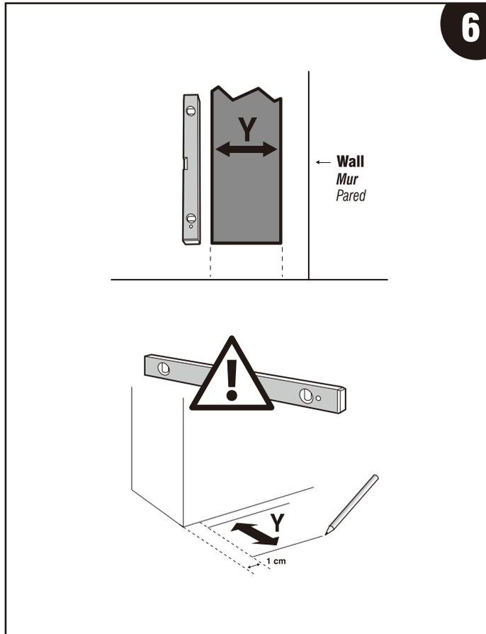
**Step 6: Install the floor guide**
