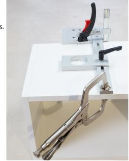
Set depth of forstner stop. Check depth stop collar set screw to assure it is tight and secure for drilling operations.
