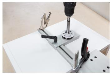
When 3/8" drill bit breaks through into puck light hole, stop drilling forward and remove the drill bit.
