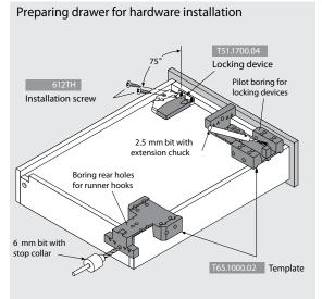
Important: Use of the T65.1000.02 template is recommended for accurate location and angle of locking device pilot holes.
