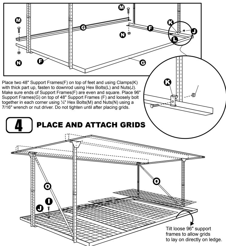
Lay 4 Wire Grids(A evenly on 96" Support Frames with grid stiffeners on the underside. Tilt loose 96" Support Frames if necessary. Tighten bolts in each corner of support frames using ½" Hex Bolts(M and Nuts(N wth a 7/16" wrench or nut driver. Fasten Wire Grids(A as shown using 4 Hex Bolts(I and Hex Nuts(J for each grid.
