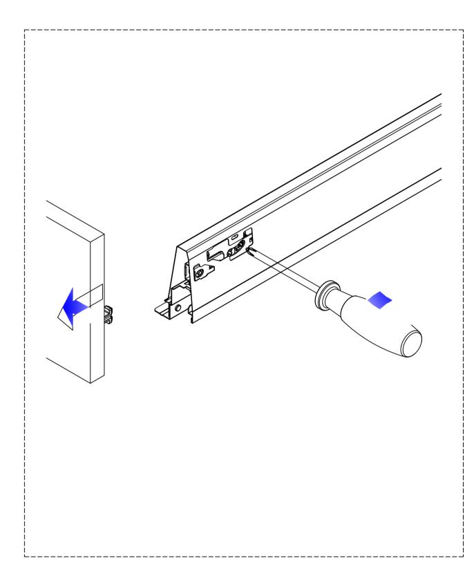
Wooden drawer front height Drawer front right adjustment: ±2mm adjustment 1mm
