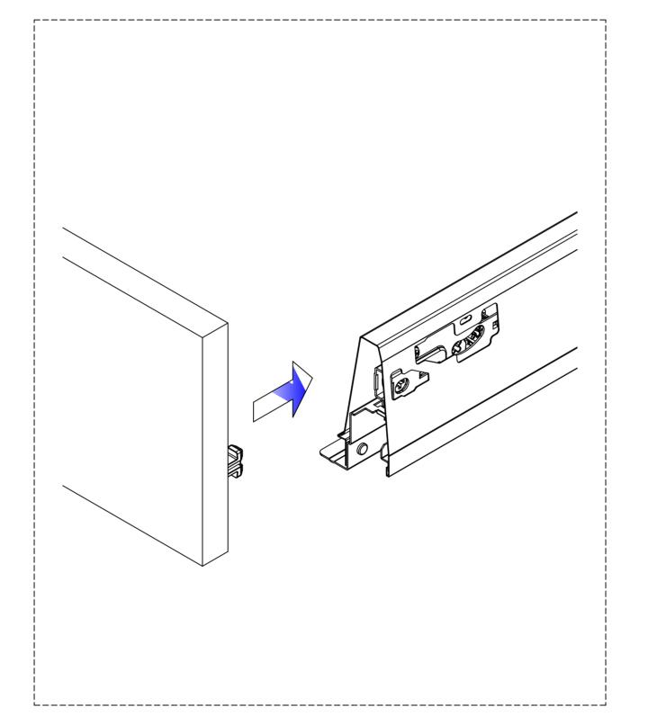
Disassemble wooden drawer front
