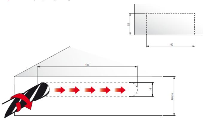
2) Drill horizontally the panel by making a second slot 100 mm wide. Hole centre 8 mm between the first and the second drilling.
