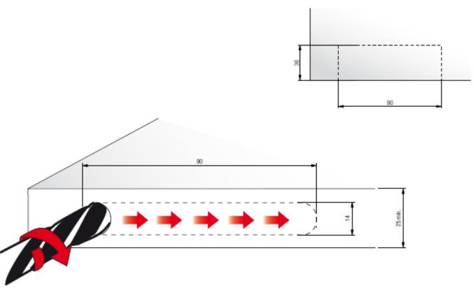
2) Drill horizontally the panel by making a second slot 90mm wide. Hole centre 5 mm between the first and the second drilling.
