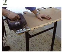
In the case of dovetailed panels, they will be squared by cutting one dovetailed end off.
