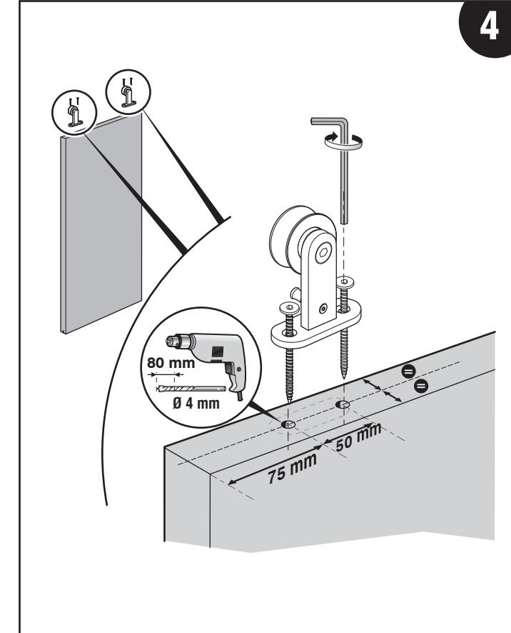
**Step 4: Attach the single bearing supports**
