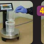
Remove liner from wall dispenser and place in 3M™ PPS<sup>™</sup> mixing cup.
