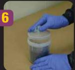
Take a lid (with built-in filter) from wall dispenser and snap onto top of 3M<sup>™</sup> PPS<sup>™</sup> cup/liner.
