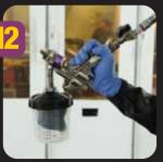
Air only needs to be bled if spraying is to be in the inverted position.
