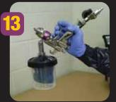
Disconnect air line, invert gun and pull trigger (full open, not partial) to return mix to gun cup before disconnecting gun.
