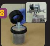
Position locking collar onto the 3M<sup>TM</sup> PPS<sup>TM</sup> cup/liner and turn until tight.
