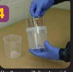
Use the cup with liner to weigh the paint according to paint manufacturer's guidelines or insert 3M<sup>™</sup> Mix Ratio Film into the cup before placing liner into cup.
