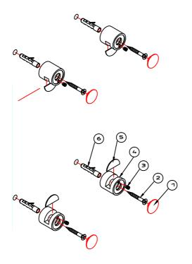
Hole diameter on the substrate; 5mm Type of screw (suggested); Dia 5mm x 40mm length
