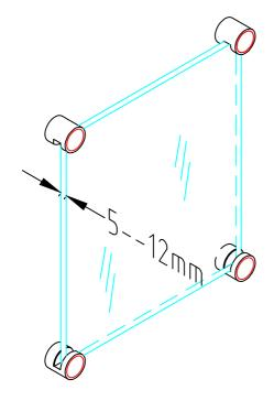
No hole in the glass sheet is required. Simply put the glass into the interior space and adjusted the it with the little screw. The space needed depends on the glass thickness (5 to 12 mm).
