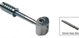
A variation of bore size of 12.5mm -13mm for Insert Screw (F) may be required for hardwoods or when drilling into end grain. Use waxing or lubrication if required to level Insert Screw flush in the material. If required countersink hole to ensure Insert Screw is flush or below surface level of material.
