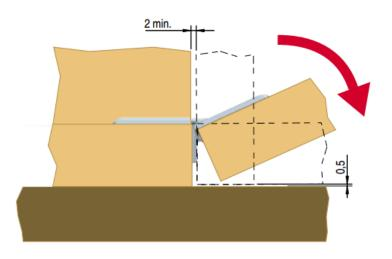
A 0,5 mm gap between the door and the platform laying underneath doesnt' interfere with the opening.
