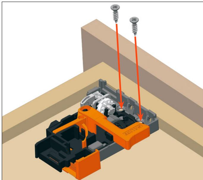
Use drilling template for accurate and level installation of the clips, see page 41.
