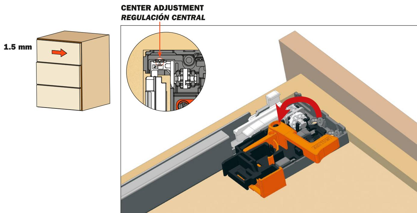
For side adjustment, it is recommended that both the adjusters on the clips are in the same direction, in order to maintain the correct alignment and function of the runners.
