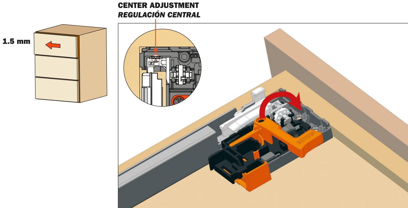
Rotate the white wheel towards the back of the drawer to adjust right.
