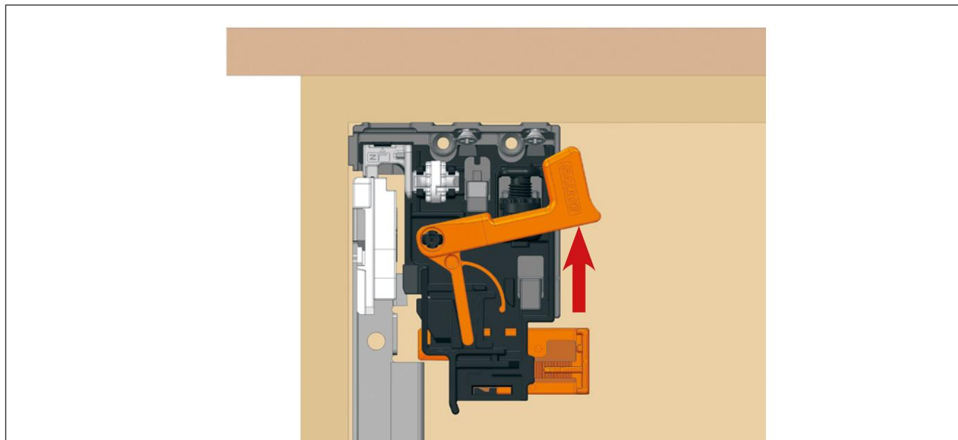
**Removal from the side:** position the hands under both sides of the drawer and press on the orange levers, as indicated in the drawing, sliding the drawer forward.
