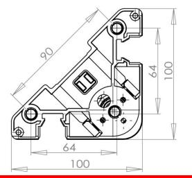
Dowels are 21mm o/c from outside edges of the 90 degree edge of the leg body.
