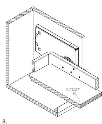
Rotate the mechanism in vertical position.
