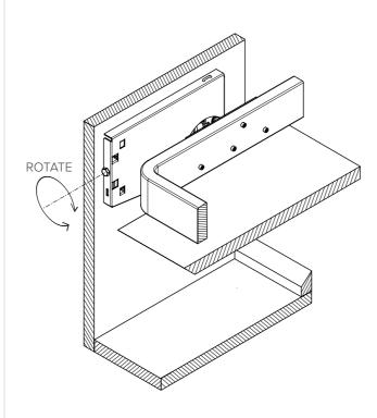
**8.**Rotate the bolt on the box's back to regulate the springs tension.
