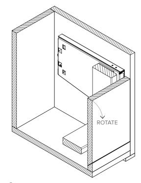
**6.**Rotate the mechanism in horizontal position.
