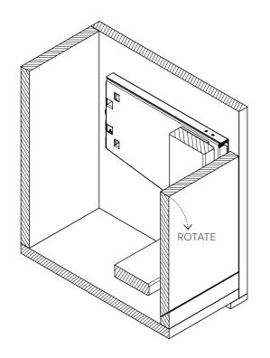
**1.** Rotate the mechanism in horizontal position.
