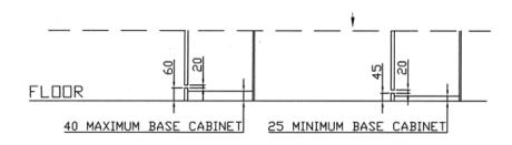
ATTENTION: FOR THE DIFFERENT DIMENSIONS OF THE BASE (25 - 40) REMEMBER TO CHANGE THE DIMENSION OF THE DOOR CABINET
