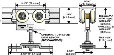
DETERMINE DOOR SIZE/HEADER HEIGHT BASED ON DIMENSIONS SHOWN IN DETAIL VIEWS AND CLEARANCE REQUIRED BELOW DOOR. INSERT C-911 HANGERS INTO TRACK AND SECURE TRACK TO HEADER
