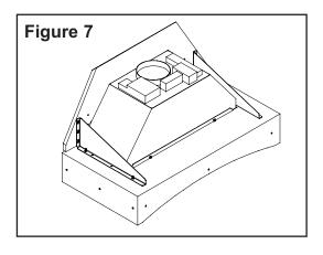
Step 8: Make all ventilation and electrical connections at this time. These must be done in accordance to all applicable building codes and requirements in your area. Duct pipe must be as close to the back wall as possible and should be 8 inch diameter or smaller.
