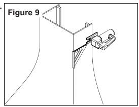
**Step 10:** Mount the Bulkhead into the Artisan Range Hood as additional support and backing for trim around the top of the Range Hood.(See figure 10).
