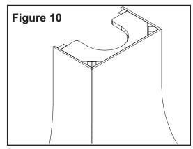
**Step 11:** Carefully position the Wood Range Hood against the wall and slide down onto the wedges. The liner should be slightly above the wood (See figure 11).
