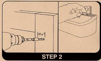
Remove the clips from the tray by disengaging spring hook as shown. Using 3/32" drill bit, prepare to drill pilot holes at locations marked in Steps 1 & 3. Wrap tape 5/16" from tip of drill bit as shown. Drill two holes at locations marked in Step 1 (do not drill deeper than front edge of tape). Mount clips at top holes using two (2) 1/2" x #6 screws (do not fasten securely).
