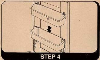
Position the tray on the clips and gently press downward to engage spring lock. This completes the installation of your Door Storage Utility Tray. To install second Door Storage Utility Tray simply repeat Steps 1-4.
