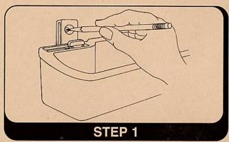
Screw-In Clip Installation - Snap one clip into the slot at each end of the tray. Hold the shelf in place and mark the screw locations using the upper holes in each clip. Note: Before marking the screw locations, you may want to use a level or tape measure to insure that the tray is straight.
