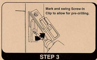
With clips in vertical position, mark bottom hole locations (swing clip to allow for drilling) and drill remaining pilot holes. Reposition the clips and securely mount top and bottom of each clip using two (2) 1/2" x #6 screws. NOTE: Use plastic screw anchors or #6-32 toggle bolts (available at your local hardware store) when installing Screw-In Clips on wallboard, plaster or very thin material.
