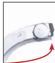
**2. Making a bushing out of a 1/2 copper pipe allowing the 3" mounting post to fit into the larger diameter accessory holes.**
