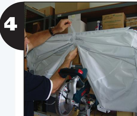
**4** Unstrap the 3 Velcro hood wraps and let the saw hood fall into position.
