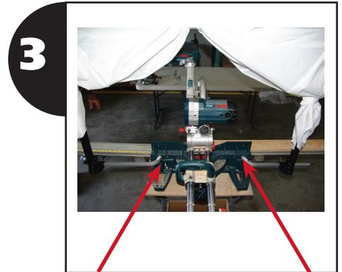
**3** Insert 1/2" roll pipe into accessory holes in mitre saw. Some accessory holes are 1/2" or 5/8" in diameter. If there is a little movement this should not be a problem.
