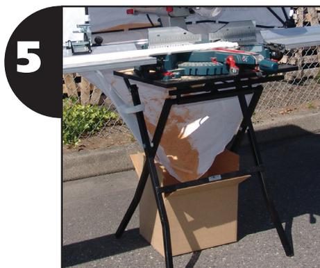
**5** We recommend that you place a trash can or box under the ChopShop Saw Hood, which allows the dust and debris to collect in one spot.
