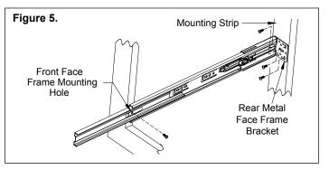
5. Extend the rear bracket until it contacts the rear vertical mounting strip. Check that both cabinet members are vertically and horizontally parallel. Mount the rear bracket using the two vertical slots. Make any necessary adjustment (Figure 5).
