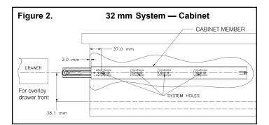
3. Use only the 32 mm system holes or the wood screw holes located at the tip of the breathing tabs. Do not use any other holes on the cabinet member for mounting (Figure 3).
