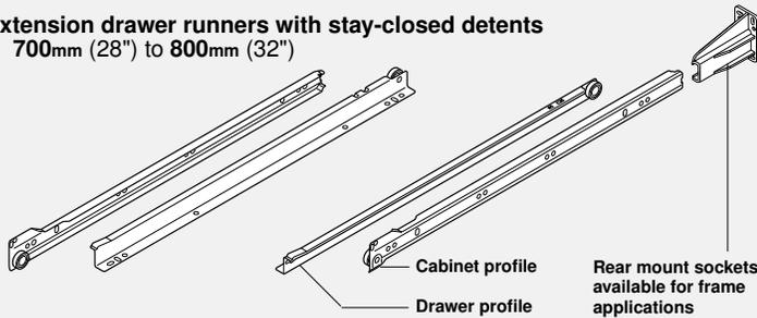
**230M** series have Blumatic self-closing action. Angled drawer and cabinet profiles create a parallel drop 3/32".
